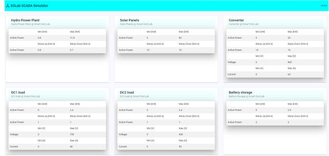
Fig. 4: SGLab SCADA simulator web interface
