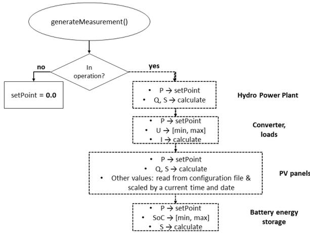
Fig. 3: Measurement generation algorithm
