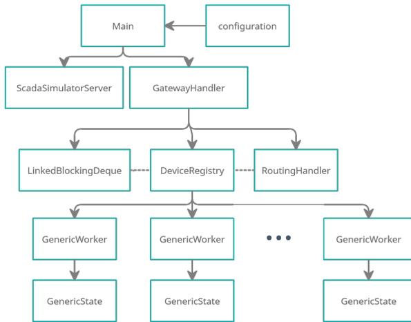
Fig. 2: SGLab SCADA simulator main modules
