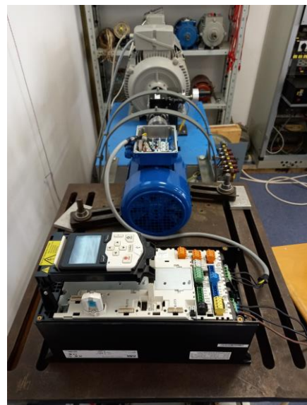
Figure 5. Frequency converter and motor
