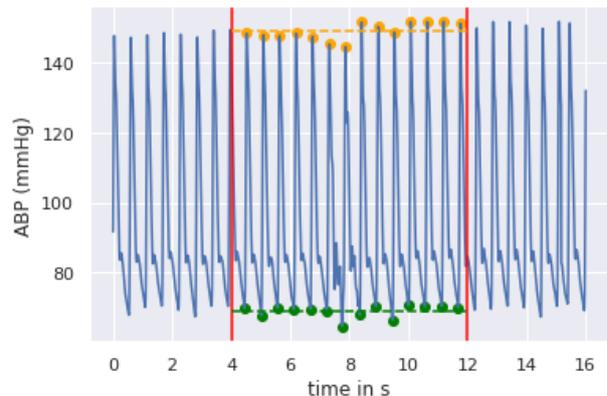
Fig. 3: Illustration of SBP and DBP extraction from ABP waveform
