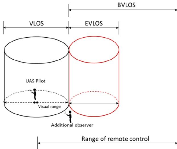
Figure 4: Separation of VLOS, EVLOS and BVLOS [9]
