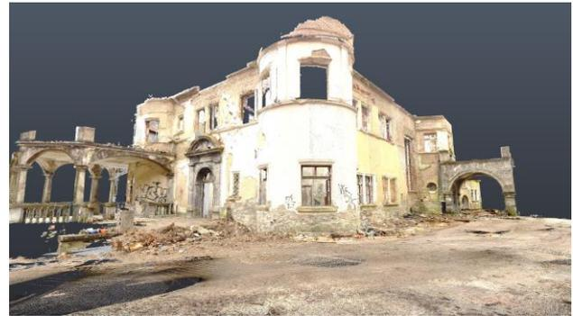
Figure 2. Denoised and filtered pointcloud of one building side
