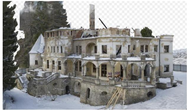
Figure 5. Denoised and filtered pointcloud connected with terrestrial and aerial photogrammetry
