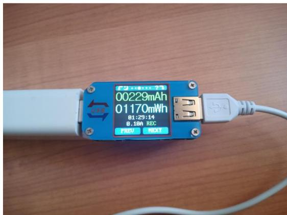
Figure 4. Measuring typical IoT device power consumption with Joy-IT JT-UM25C device using recording of charging/discharging mode
