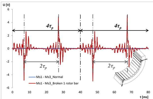
Figure 8. Voltage difference between measuring coils Ms1 and Ms3 for normal (blue waveform) and for one broken rotor bar (red waveform).
