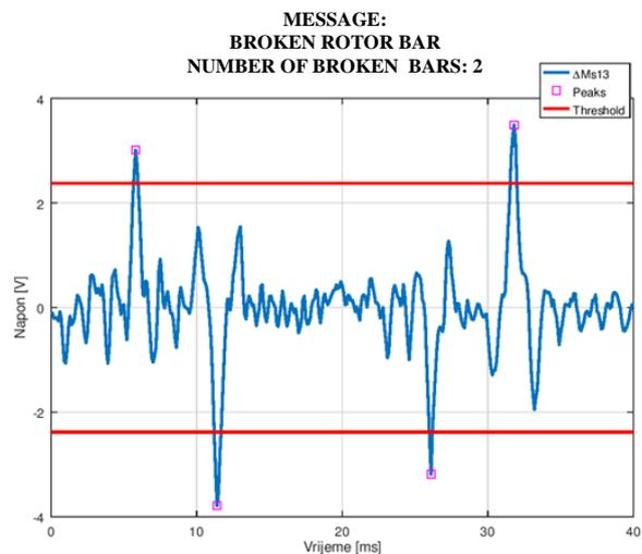
Figure 14. Algorithm output message – broken two rotor bars
