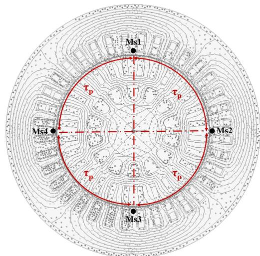
Figure 3. Distribution of the magnetic field with position of the measuring coils.
