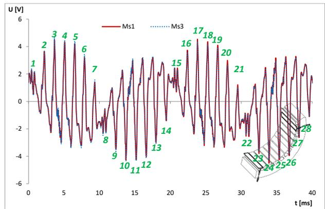
Figure 5. Impact of the squirrel-cage rotor bars on the induced voltage waveform in measuring coils.
