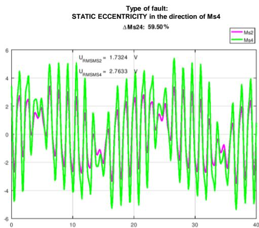
Figure 17. Algorithm output message – occurrence of static eccentricity in the direction of the measuring coil Ms4
