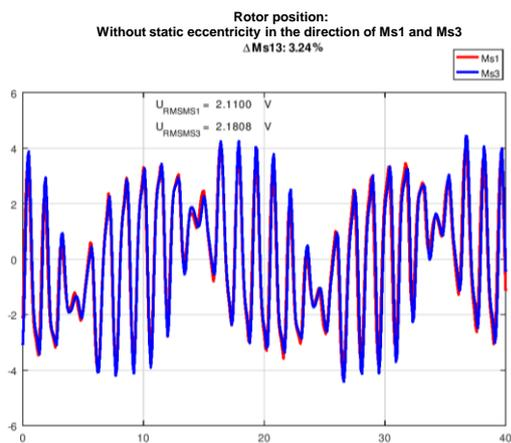
Figure 16. Algorithm output message – without the presence of static eccentricity
