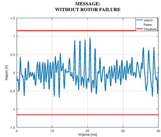
Figure 12. Algorithm output message – without rotor failure
