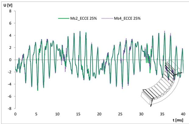
Figure 7. Comparison of the induced voltage waveform in the measuring coils for the static eccentricity amount 25% of the air gap (a shift in the + y axis): Ms2 and Ms4 diametrically spaced.
