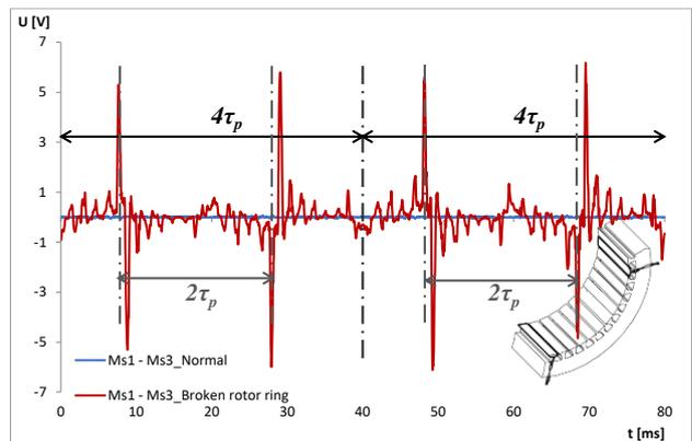
Figure 10. Voltage difference between measuring coils Ms1 and Ms3 for normal (blue curve) and for broken rotor ring (red curve).
