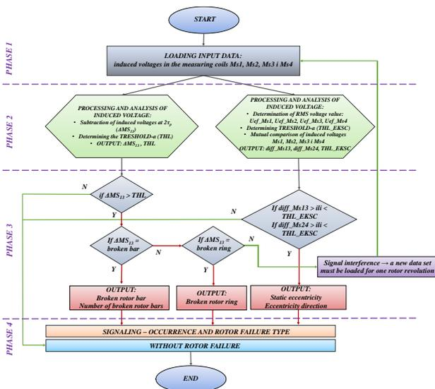
Figure 11. Flowchart of the smart and advanced algorithm for reliable faults detection and their mutual recognition.
