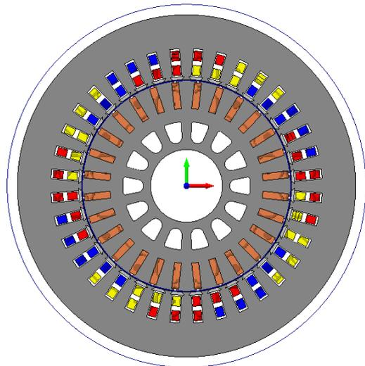
Figure 2. 2D FEM model of induction motor.
