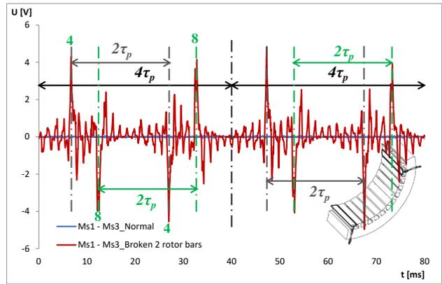
Figure 9. Voltage difference between measuring coils Ms1 and Ms3 for normal (blue curve) and for two broken rotor bar (red curve).
