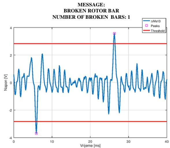
Figure 13. Algorithm output message – broken one rotor bar
