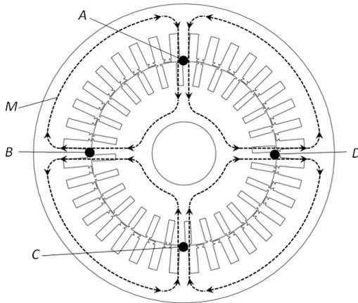
Figure 1. Presentation of the magnetic field line distribution along with locations for installation of measuring coils for magnetic field measurement [24].
