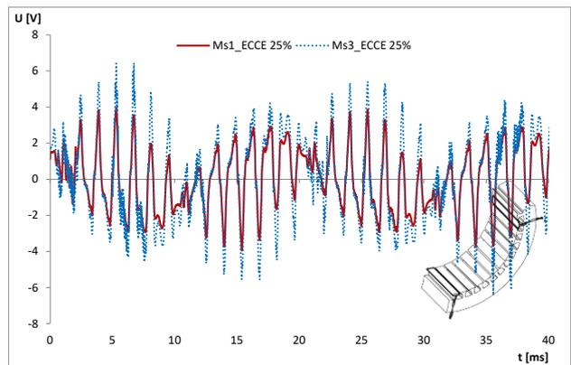
Figure 6. Comparison of the induced voltage waveform in the measuring coils for the static eccentricity amount 25% of the air gap (a shift in the + y axis); Ms1 and Ms3 diametrically spaced.
