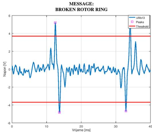
Figure 15. Algorithm output message – broken rotor ring
