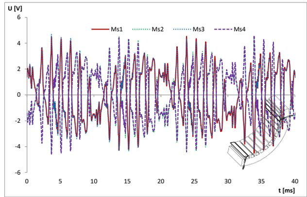
Figure 4. Induced voltage waveform in the measuring coils Ms1, Ms2, Ms3 and Ms4 – normal condition.
