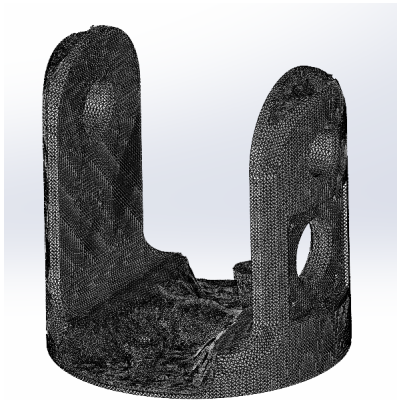
Figure 2. Topologically optimized shoulder in SolidWorks
