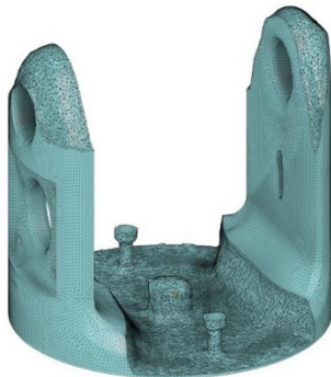
Figure 3. Topologically optimized shoulder in Fusion 360
