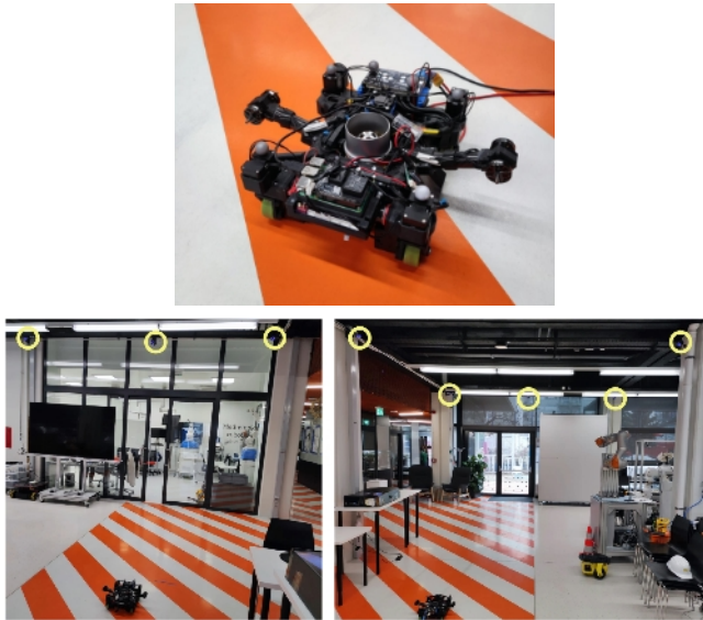
Fig. 6. Photo of the experimental set-up of the mobile robot and OptiTrack system.
