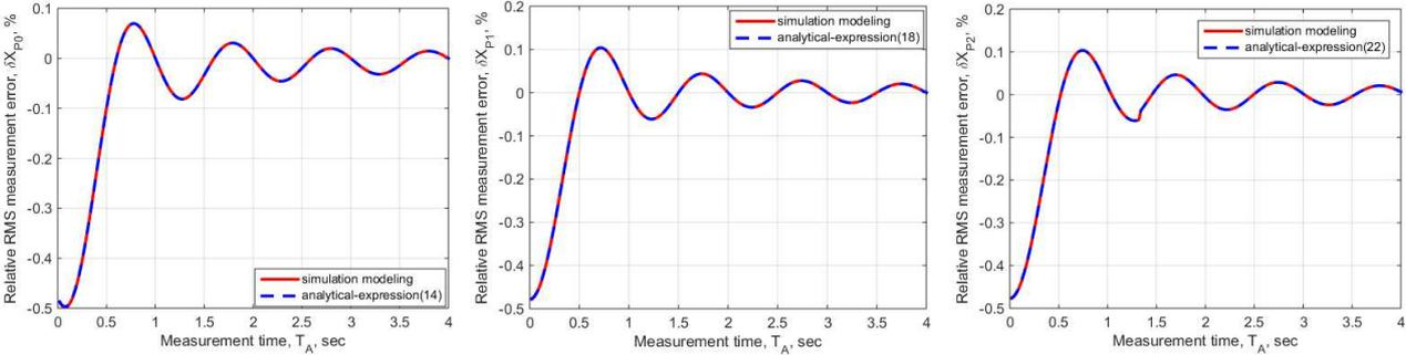
Figure 3. Dependence of the RMS measurement error of a sinusoidal signal on the total measurement time. From left to right: zero-order approximation polynomial, first-order polynomial, second-order polynomial.
