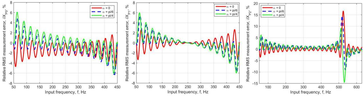
Figure 1. Dependence of the RMS measurement error on the input signal frequency for different values of the initial phase of the measured sinusoidal signal. From left to right: zero-order approximation polynomial, first-order polynomial, second-order polynomial.
