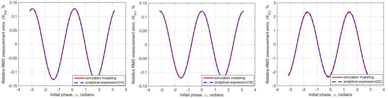
Figure 2. Dependence of the RMS measurement error on the initial phase of the measured sinusoidal signal. From left to right: zero order polynomial, first order polynomial, second order polynomial.
