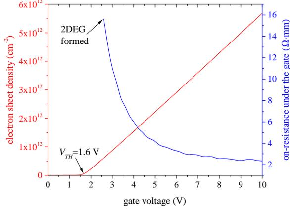
Fig. 3: Gate voltage dependence of the electron sheet density and on-resistance in the region under the gate. The threshold voltage of  $V_{TH} = 1.6$  V matches the experimentally obtained value [22].
