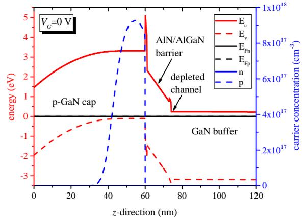
Fig. 2: Band diagram and carrier concentrations under the gate of the simulated HEMT structure at  $V_G = 0$  V. The presence of the p-GaN cap layer depletes the 2DEG in the channel and results in enhancement-mode operation.
