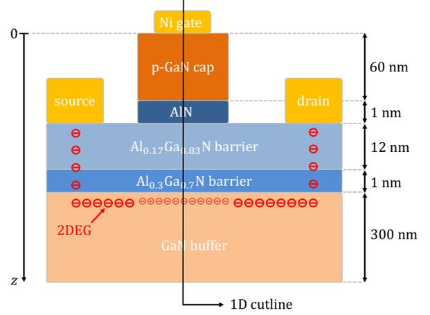
Fig. 1: 2D cross-section of the studied composite-barrier HEMT with a p-GaN cap. The 1D calculations are performed along the cutline in the  $z$ -direction.
