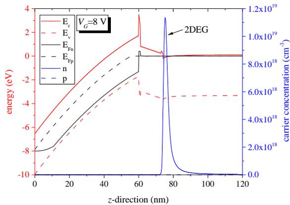
Fig. 4: Band diagram and carrier concentrations under the gate of the simulated HEMT structure at  $V_G = 8$  V. The position-dependent quasi-Fermi levels are obtained by solving the continuity equations for both types of carriers.
