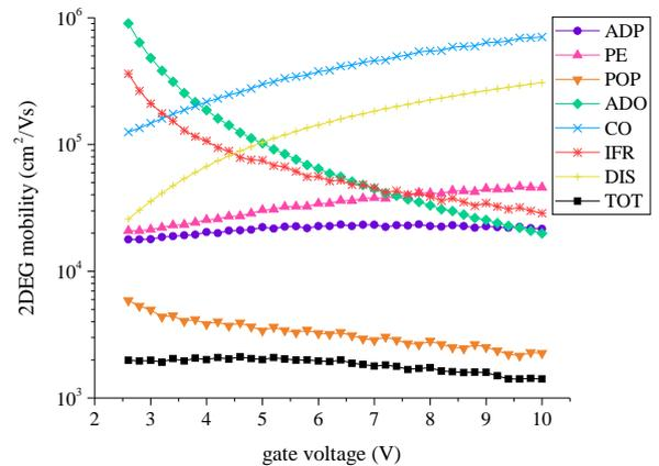
Fig. 5: Gate voltage dependence of the room-temperature 2DEG mobility limited by different scattering mechanisms for the GaN HEMT in Fig. 1. The POP-limited mobility is the dominant factor determining the total mobility, which shows a slight decrease due to stronger confinement at high gate voltages.
