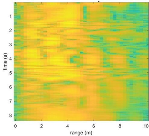
Fig. 3. Range diagram for a stationary object in indoor environment (horizontal polarization).
