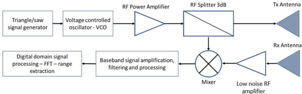
Fig. 1. FMCW radar principal components and layout
