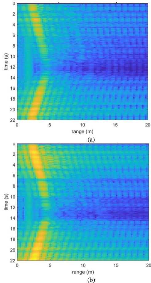
Fig. 6. Range detection for a moving object; (a) horizontal polarization with CCD, (b) vertical polarization with CCD.
