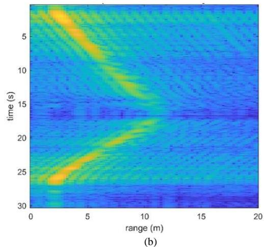
Fig. 4. Range detection (horizontal polarization) for a moving object; (a) without CCD, (b) with CCD.
