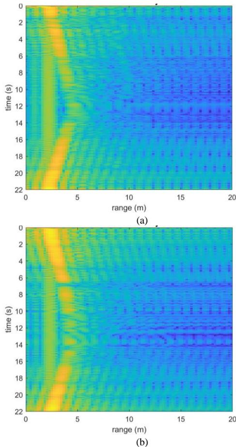
Fig. 5. Range detection for a moving object; (a) horizontal polarization without CCD, (b) vertical polarization without CCD.
