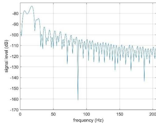
Fig. 2. Output from the IFFT block in FMCW processing showing the detected beat frequencies in baseband for measurement in the lab environment.
