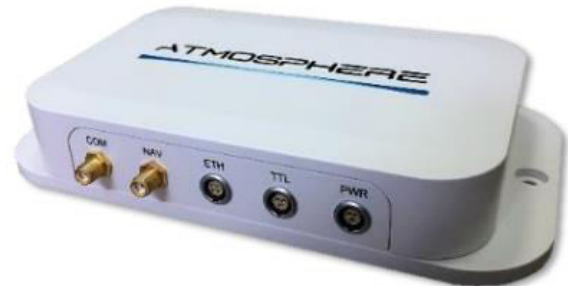
Figure 1: PLANET connectivity solution flown onboard the UAV (Source: own)
