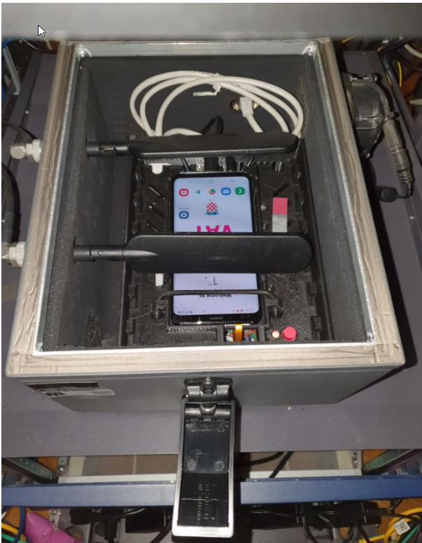
Figure 2. Shielded box with the mobile probe inside
