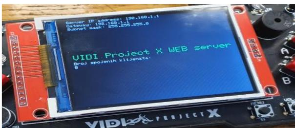
Figure 8. VIDIX micro server. Display of server network settings and the number of connected wireless clients. Source: vidilab.com [7]
