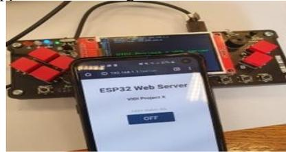
Figure 9. Mobile application that turns on/off the VIDIX LED
