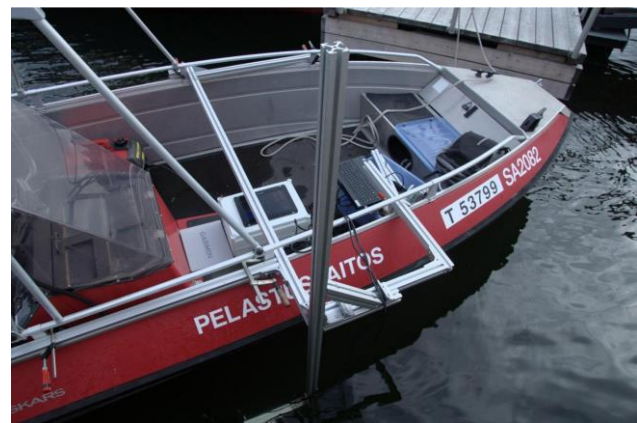
Figure 1 Data collection devices installed into the boat of the rescue department. Power to the laptop and to the sonar is taken from the small gasoline generator. The system is designed to be easy to fit to most of the small boats without any holes or other permanent marks [6].
