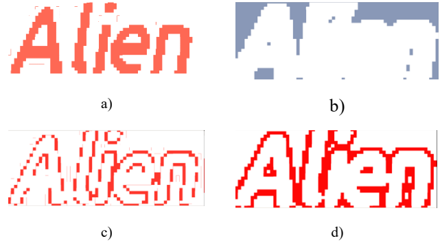
Figure 3. Segmentation of the image shown in Fig. 2 using k -means algorithm in four clusters.
